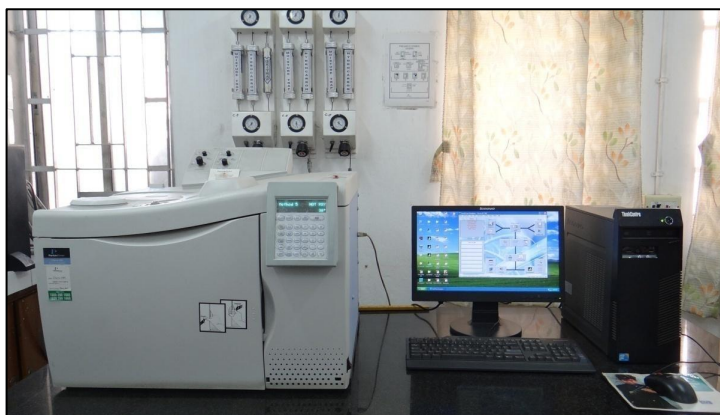
Gas Chromatograph (GC) (Perkin Elmer; CLARUS 480).
