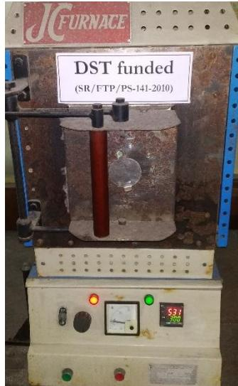
High temperature muffle furnace
