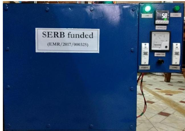
Tube furnace for high temperature measurement
