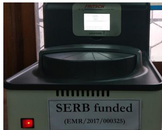
**Planetary Ball Mill (Fritsch, P-7)**
